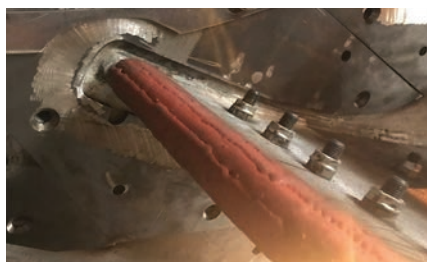
Bolts attaching a wearplate to an impeller
