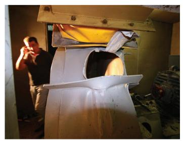
replacement for a glass chiller fan on the point of failure.
