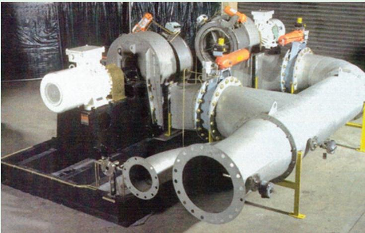
*Halifax Fan assembly designed for hazard environment*
