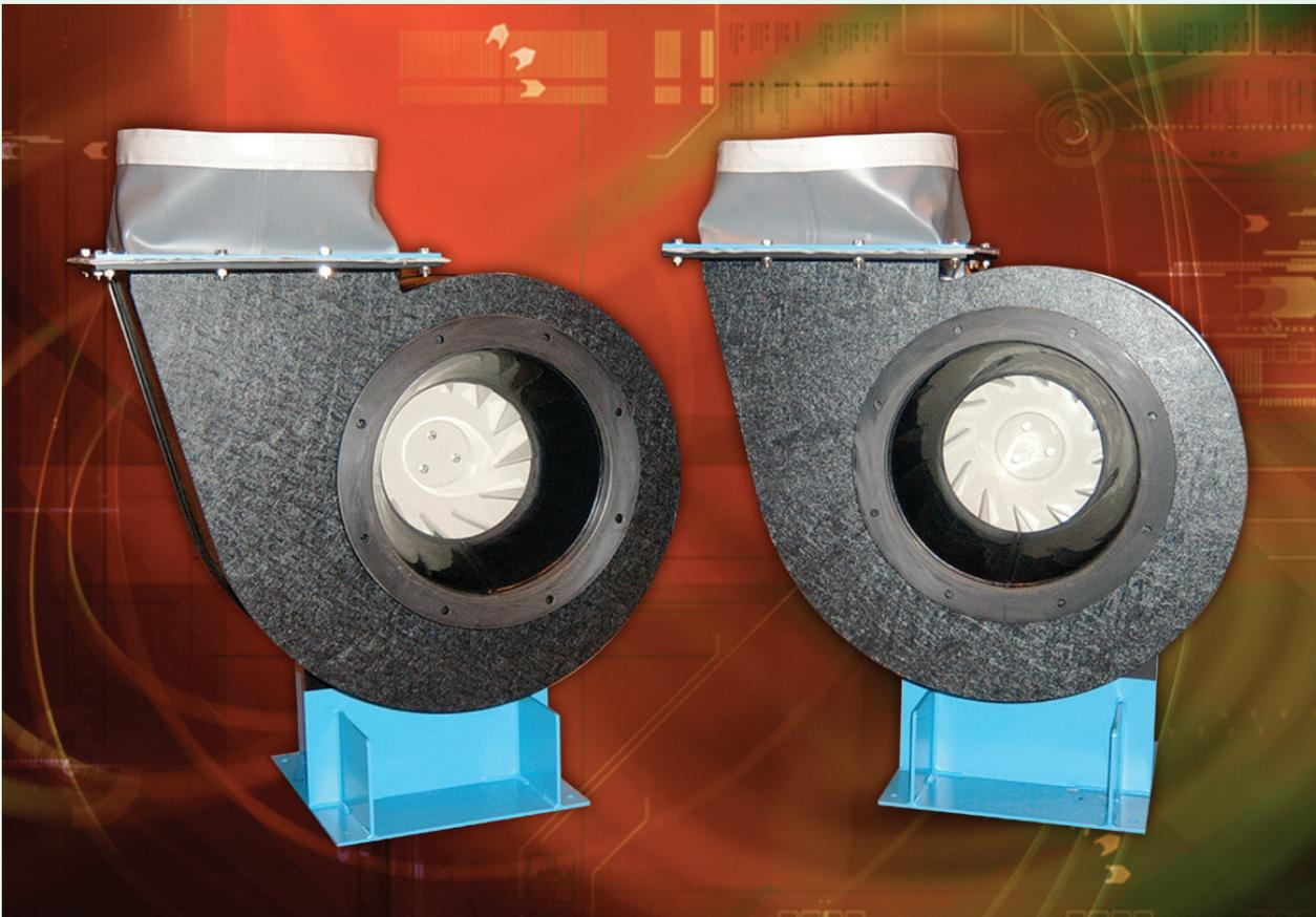
The new range is based on the existing fan range, covers a wide range of physical sizes and will offer duties up to 50,000m<sup>3</sup>/hr and pressures up to 5000Pa. Fan casings are fabricated from co-polymer black poly-propylene, embossed on the exterior surface to increase durability and scratch resistance, with the impeller removable from either the inlet or
